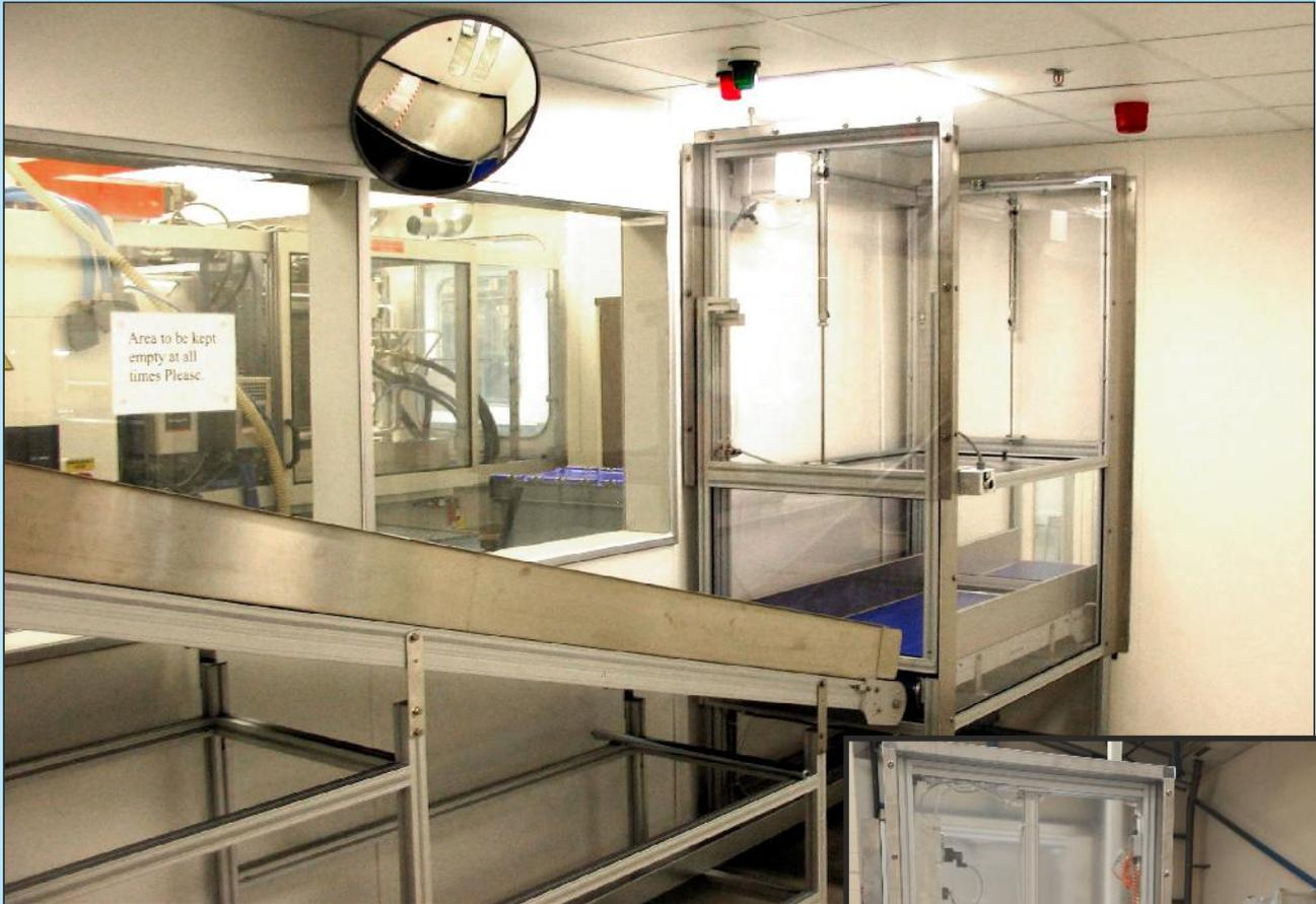
Our clean room air lock has integral conveyors, sealed vertical sliding doors.
